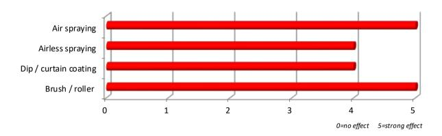
UNIQ®FOAM 132 S is medium to strong defoamer to be used in clear coatings as well suitable for pigmented coating systems. Due the chemical structure the product will not cause turbidity, but will give good air-release and macro defoaming properties. Also very well suited for PE primers remaining high clarity and transparency. The product is well suited for spraying applications.
