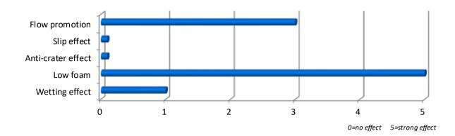
UNIQ FLOW 392 S is a polyacrylate surface active agent for solvent based applications especially suitable for baking systems. It promotes leveling, has defoaming effect (particularly for micro foam), and is effective for very short baking times. Suitable for roller application, conventional spraying application, and airless/airmix applications.
