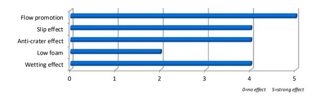
UNIQ®FLOW 415 S is a highly effective silicone additive, provides a strong reduction of surface tension. Offers good wetting of critical substrates. In pigmented systems it can prevent the formation of Bénard cells and improve leveling. UNIQ®FLOW 415 S improves the acceptance of dust and spray mist and increases surface slip. It reduces air draft sensitivity in wood and furniture coatings.
