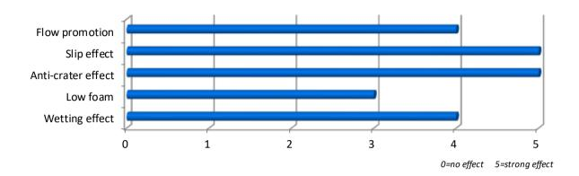
**UNIQ** FLOW 440 U is modified polyether polysiloxane leveling agents. The product can offer strong reduction of surface tension and improves wetting effect and anti-crater effect of substrate. Meanwhile, it shows the good performance of fast leveling.
