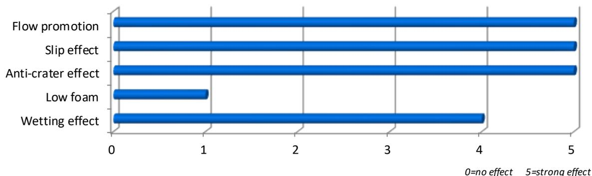
**UNIQ<sup>®</sup> FLOW 493 U** is modified polyether polysiloxane leveling agents. The additive gives strong surface tension reduction properties in coatings. The substrate wetting is improved and therefore can also act as an anti-crater agent. **UNIQ<sup>®</sup> FLOW 493 U** gives strong surface slip and can help to increase the gloss. In aqueous systems it improves the anti-blocking properties
