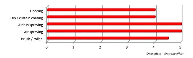
UNIQ® FOAM 158S is a Silicone free polymeric defoamer suited for solvent-free-, radiation-curing wood- and industrial coatings, printing inks and adhesives. It an be used in pigmented and clear coat systems applicable in every coating layer without effecting the intercoat adhesion and recoatability. Specially suited for epoxy resin, but also very good performances in polyurethane resin types.
