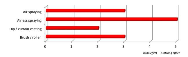
**UNIQ** FDAM 175 S is especially effective in wood and furniture coatings based on glossy polyester, paraffin polyester, and in radiation curable polyester. The additive allows curtain coaters to maintain curtain stability even when only thin layers are applied. When using non-pigmented systems, a slight turbidity may be visible over dark wood. Good results were also found with epoxy systems.
