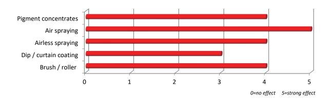
UNIQ® FOAM LP2507 is a strong defoamer/anti-foam based on organic polymers, this product can be used for grinding and spraying conditions. Working well against macro-foam, but delivers also strong micro-foam destroying properties. It is well suited for all water based systems and pigment concentrates.
