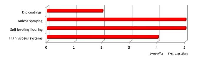
**UNIQ** FOAM P-575 is a strong anti-foam and air-release agent especially suitable for ambient-curing plastic systems and adhesives and sealants, especially for epoxy and PU based resin systems. The additive furthermore helps to improve the leveling and avoids pinholing or popping.
