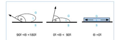
At a contact angle  $> 90^\circ$  no wetting takes place and the droplet keeps its spherical shape.
