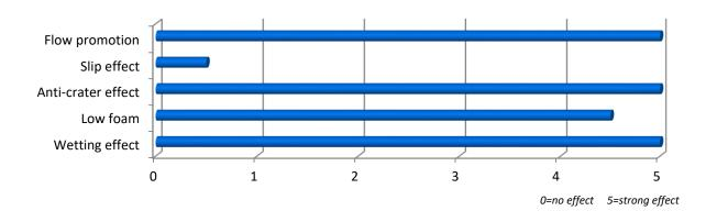
**LNIC**<sup>®</sup>**FLOW 483 U** is a silicone type wetting and leveling agent, can be used in various water based, solvent based and UV coatings. Excellent substrate wetting efficiency, effectively preventing edge crawling, good anti-foam, defoaming performance. The product can be used to from primer to topcoat without effecting the intercoat adhesion.
