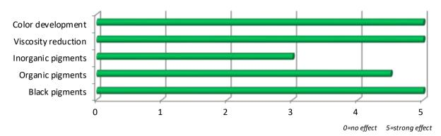
UNIQ®SPERSE 580 U is a wetting and dispersing additive for water based and solvent free applications. Suitable for industrial, automotive coating and resin free pigment concentrates.
