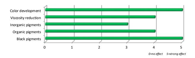
**UNIQ** \*\*SPERSE 680 **U** is a wetting and dispersing additive for water based or solvent based applications. The dispersant is especially developed for the grinding of carbon black to give excellent jetness development. Also very well suited for inorganic or organic pigments and resin free pigment concentrates.
