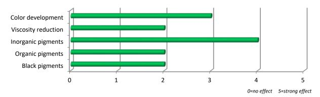
UNIQ®SPERSE P-160 is a wetting and dispersing additive in unsaturated resin systems and adhesives. The additive prevents the flooding/floating and settling of pigments and fillers in epoxy and VE/UP-based laminates. Reduction in the flooding/floating of colored pigments in gel coats.
