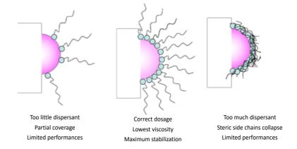
As a general rule, 2-2.5 mg of polymeric dispersant, per square meter of pigment surface area will be close to the optimum amount required.
